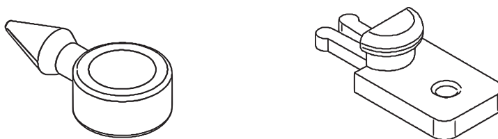
Figure 2 Left: straight peg. Right: anchor peg.
